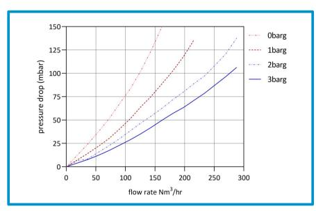
Air flow vs pressure drop at various pressures for a 10 inch BPFM, 0.2 µm zPTFE membrane filter cartridge
