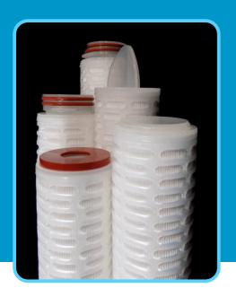
BorsoPTFE-M filter cartridges are manufactured with a unique structure incorporating a PTFE membrane with a reduced resistance to flow (zPTFE), that allows a high flow with minimal pressure drop while ensuring full retention of contaminant bacteria. A high-temperature resin is used for constructing the hardware to ensure that the filter can withstand high temperature steaming without distortion or damage.
