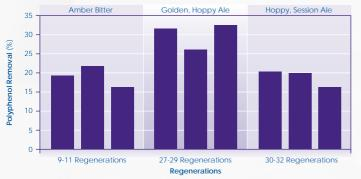
A number of different types of beers were processed through a scaled down BorsoPVPP in the form of a small module. The selected flow rate gave an adsorbent/beer contact time of 25 seconds. For every 6 litres of beer processed, the system underwent in-situ regeneration with caustic and reverse-osmosis water. A nitric acid wash was added every 3rd regeneration cycle to negate any effects of beer stone formation.
