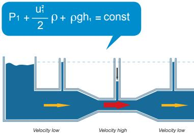
Velocity low Static pressure high Velocity high Static pressure low
